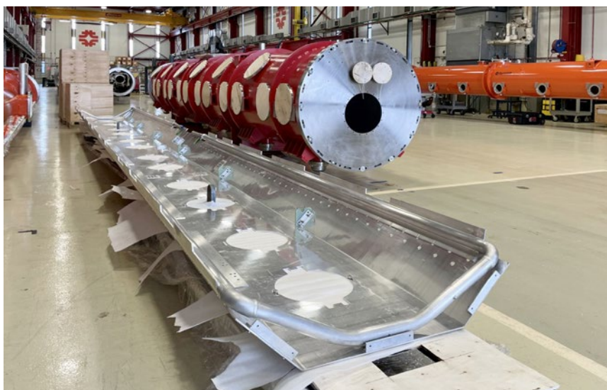
The vacuum vessel and strongback for the prototype HB650 cryomodule in the Industrial Center Building.
