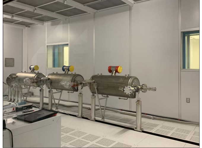
Three of six cavities in the prototype HB650 cryomodule string after installation of high power RF couplers, interconnect bellows, and cold-to-warm transition. This is the first of its kind string, assembled in a new cleanroom facility. Credit: Saravan Chandrasekaran
