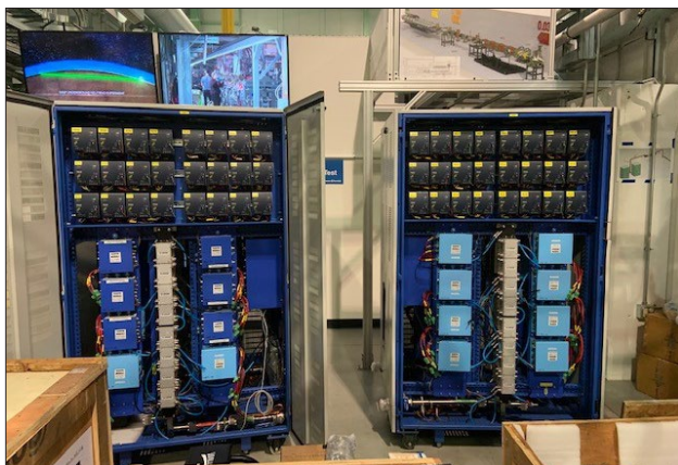
40kW RF amplifier prototype is being assembled in CMTF.
